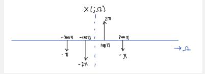
(b) For this part, there is actually a trick from going from the CTFT to the DTFT explicitly, and so plotting  $X(j\Omega)$  first (previous part) and then plotting  $X(e^{j\omega})$  would be easier. Then we can plot this simply by re-scaling the axis from part (a) with  $\omega = \Omega T$ , where T = 1/500 seconds. However, for now, we will just compute x[n] = x(nT) and plot the DTFT. This will be
