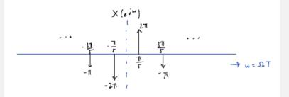
(c) To get y[n], our input signal x[n] goes through an ideal low pass filter with cutoff frequency  $\omega_c = \frac{2\pi}{5} \frac{\text{rad}}{\text{sec}}$ . I think plotting first and then stating the resulting equation would be easier:
